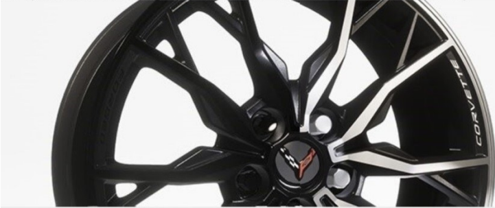
20-spoke bright machined-face forged aluminum (19" x 8.5" front and 20" x 11" rear)
