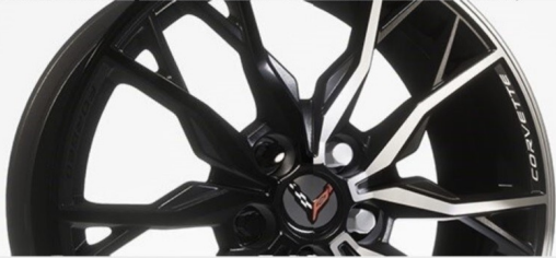
20-spoke bright machined-face forged aluminum (19" x 8.5" front and 20" x 11" rear)
